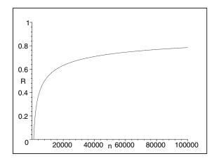
Fig. 3. The ratio  $R = C_d/C_d^{(u)}$  as a function of number of nodes *n*. Note that the ratio approaches 1 rather slowly. This example uses Q = 0.99 and  $\lambda d = 0.2$ .
