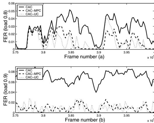
Fig. 5. Time variation of the received voice frame error rate: (a) at offered load 0.8; (b) at offered load 0.9.
