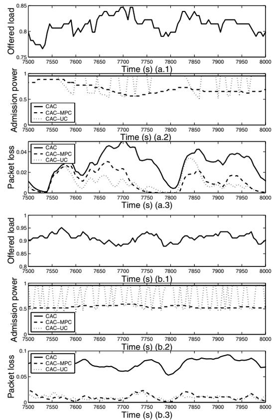
Fig. 4. Time variation of offered load, power threshold and packet loss rate for CAC, CAC-MPC and CAC-UC: (a) at offered load 0.8; (b) at offered load 0.9
