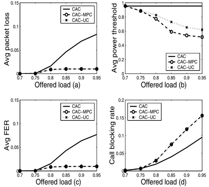
Fig. 2. Performance metrics of CAC, CAC-MPC, and CAC-UC as a function of offered load: (a) average packet loss rate; (b) average power threshold; (c) average frame error rate; (d) average call blocking rate.
